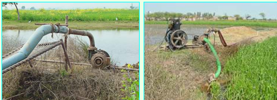
Fig. 7. Dewatering of wheat fields by pumps driven by (a) electric motor and (b) diesel engine
